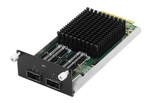
LREM7100PF-2QSFP+ is a dual-port 40G mezzanine fiber Ethernet network card developed by Shenzhen Lianrui Electronics Co., Ltd. based on the Intel XL710 chip solution. The adapter card adopts a mezzanine structure, which is convenient for use on security platforms such as firewalls and gateways. At the same time, it provides unparalleled features for device and network virtualization functions to meet the needs of data transmission.
