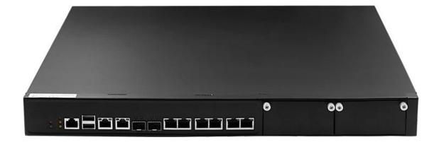
The router's default LAN0 IP address is configured as <a href="https://10.3.3.10/16">https://10.3.3.10/16</a>. You can access the router's web interface using browsers such as Chrome or Firefox.
