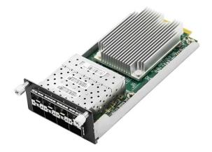
LREM3503PF-8SFP is a PCI Express x8 eight-port fiber mezzanine Gigabit Ethernet network adapter developed by Shenzhen Lianrui Electronics Co., Ltd. based on the Intel I350 main control solution. It is used in firewalls, gatekeepers, data monitoring and other data. In terms of transmission, it adapts to non-stop operation around the clock.
