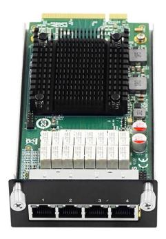
LREM3503BP-4T is a PCI Express x8 Quad-port mezzanine gigabit BYPASS Ethernet network adapter developed by Shenzhen Lianrui Electronics Co, Ltd. on the basis of Intel I350 master control scheme. The adapter is used in a mezzanine structure, and is applied to data transmission such as firewalls and gateways to adapt to non-stop operation around the clock.
